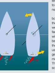
Having stopped our boat and felt its windage, the second exercise we teach skippers familiarizing themselves with a new boat's behaviour is to turn the boat through 180° using forward, reverse gears and the helm from motoring slow ahead. This mimics the common
