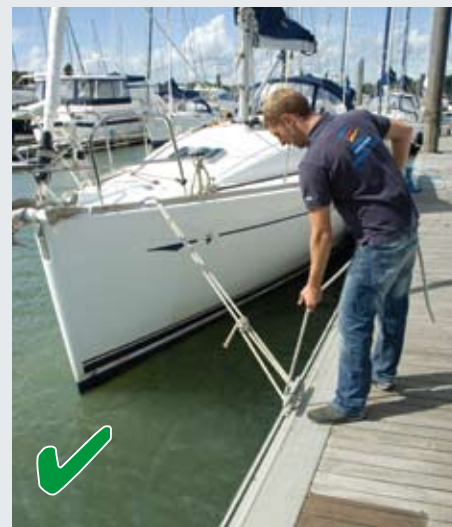
When preparing to slip, run the slipping lines before you undo the mooring warps
