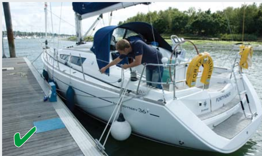
When slipping lines try not to share slipping points and fairleads. At the stern the genoa winches can often provide a useful extra slipping point.
