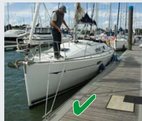
A wide triangulated slip, with incoming line not sharing a fairlead with the outgoing one and without excessive amounts of line to slip.
